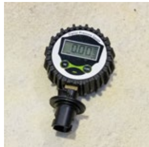
Manometer for checking the air pressure.
